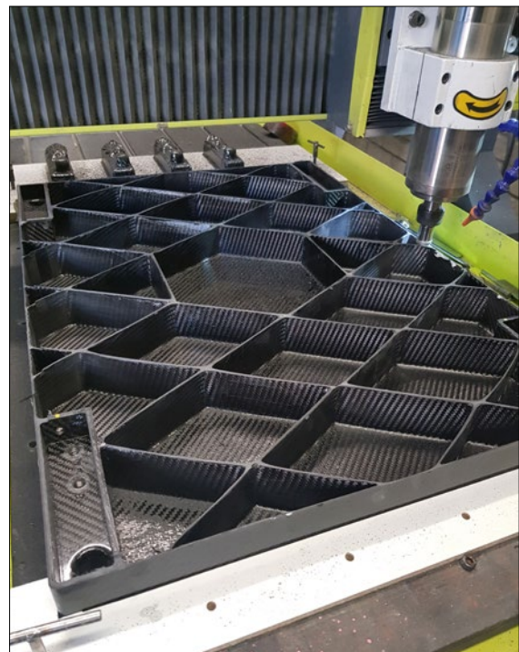
Innervations C-Force carbon fibre performance force platform – top. Prototype by Composites Components. Image courtesy G. Oldfield
