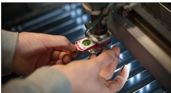
Top Left. Aquatic Leisure Technologies - Fit out bay Left. Electrical engineer repairs a laser cutting head on large CNC computer numerical control printing and cutting machine Above. Finishing a composite part.
